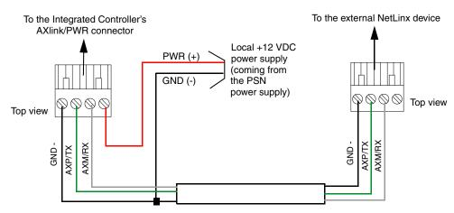
FIG. 9 4-pin mini-Phoenix connector wiring diagram (using external power source)
